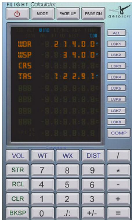
Now we only need to enter the course we took from the charts. So we enter 169 on the keypad. Well see that appear on the scratchpad, the bottom most line of the screen. If you make a mistake just use the [BKSP] to clear the display.
