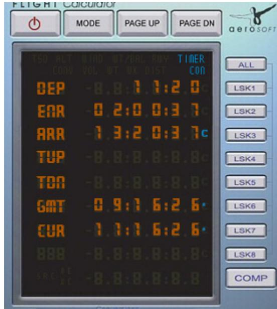
As we like to know how much fuel we will use we copy the time enroute to the scratchpad and select the TSD (Time-Speed/Distance) mode and the F (Fuel) sub mode. It's clear that we need the time enroute and the fuel flow.
