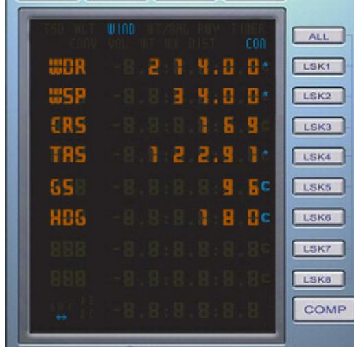
As we need the Ground Speed for the other calculations we copy that back to the scratchpad by clicking the [LSK5] line. Now we have to select a new mode, so we click [MODE], and select TSD (Time/Speed/Distance) and TPS (Time/Speed).
