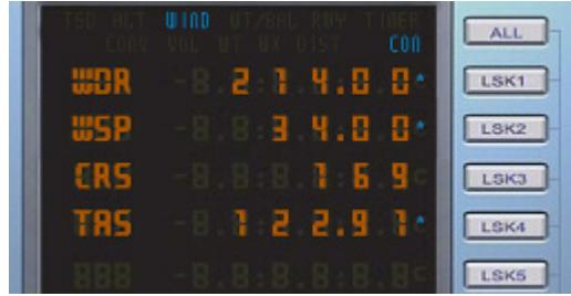
With all data entered we press the [COMP] key to do the calculations. We see the results appear on the [LSK5] and [LSK6]. We now know that we will have to fly a heading of  $180^\circ$  to stay on the  $169^\circ$  course (the wind is on our right front). We'll end up with a ground speed of 96 knots. So we'll loose a lot of speed due to the wind. But this is an old lady and we can't go faster. As long as we got enough fuel we'll be fine.
